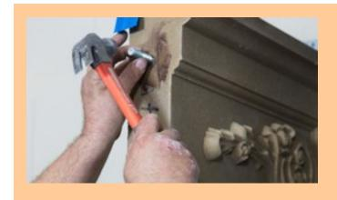
The excess All-Thread cut from the corbel and header return can be used as your pins for the header to the header return.
